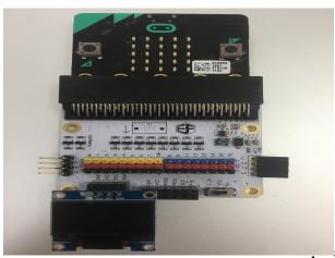
Put the micro:bit into the Breakout Board and put the OLED onto any of the 4 holes seen at the bottom of the Breakout Board.
